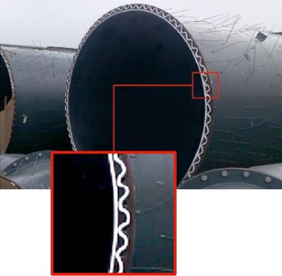
Complete the gasket by placing the joint sealant over the first skived end, extending the joint sealant at least ~15 mm (1/2") beyond the top of the skive ramp, and cutting the end square. Press out any gaps between the two gasket layers at the first skive ramp.
